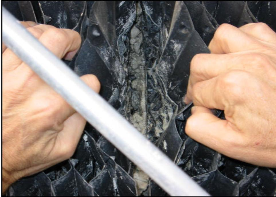
Media condition after 8 hours **OXIDE** treatment showing softening of scale deposits. Note difficulty in separating media.
