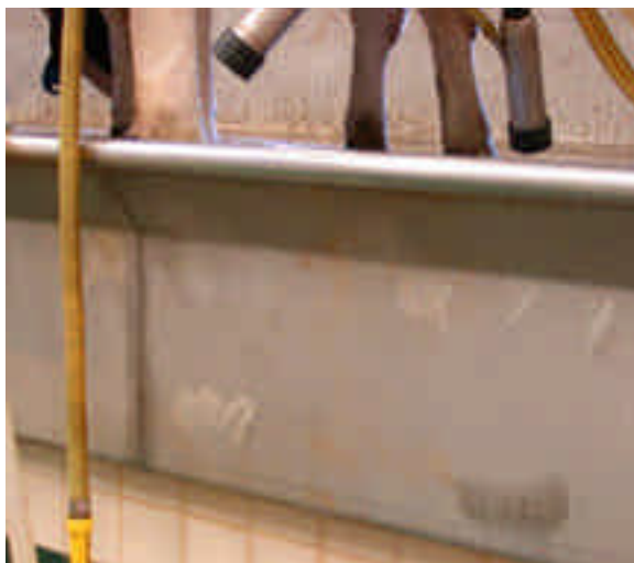
60 days after treatment, scale was entirely removed and no new scale was formed.
